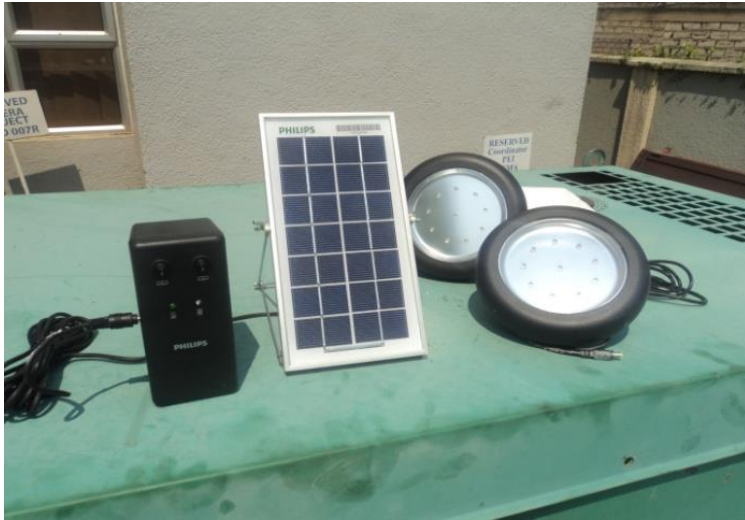
FIGURE 4-3: SOLAR LIGHTS WITH FOUR ESSENTIAL COMPONENTS
